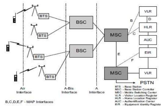
**Fig .1. Outline of GSM network architecture**
